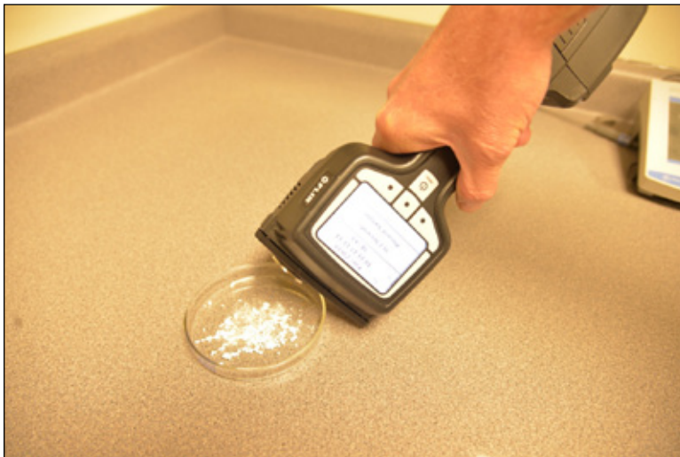
Fig. 2. Vapor-based sample collection and analysis (Source: FLIR, 2018).
