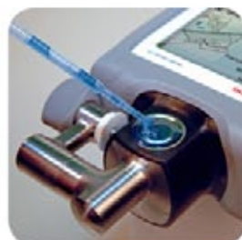
Liquids containment well prevents chemicals from spilling.
