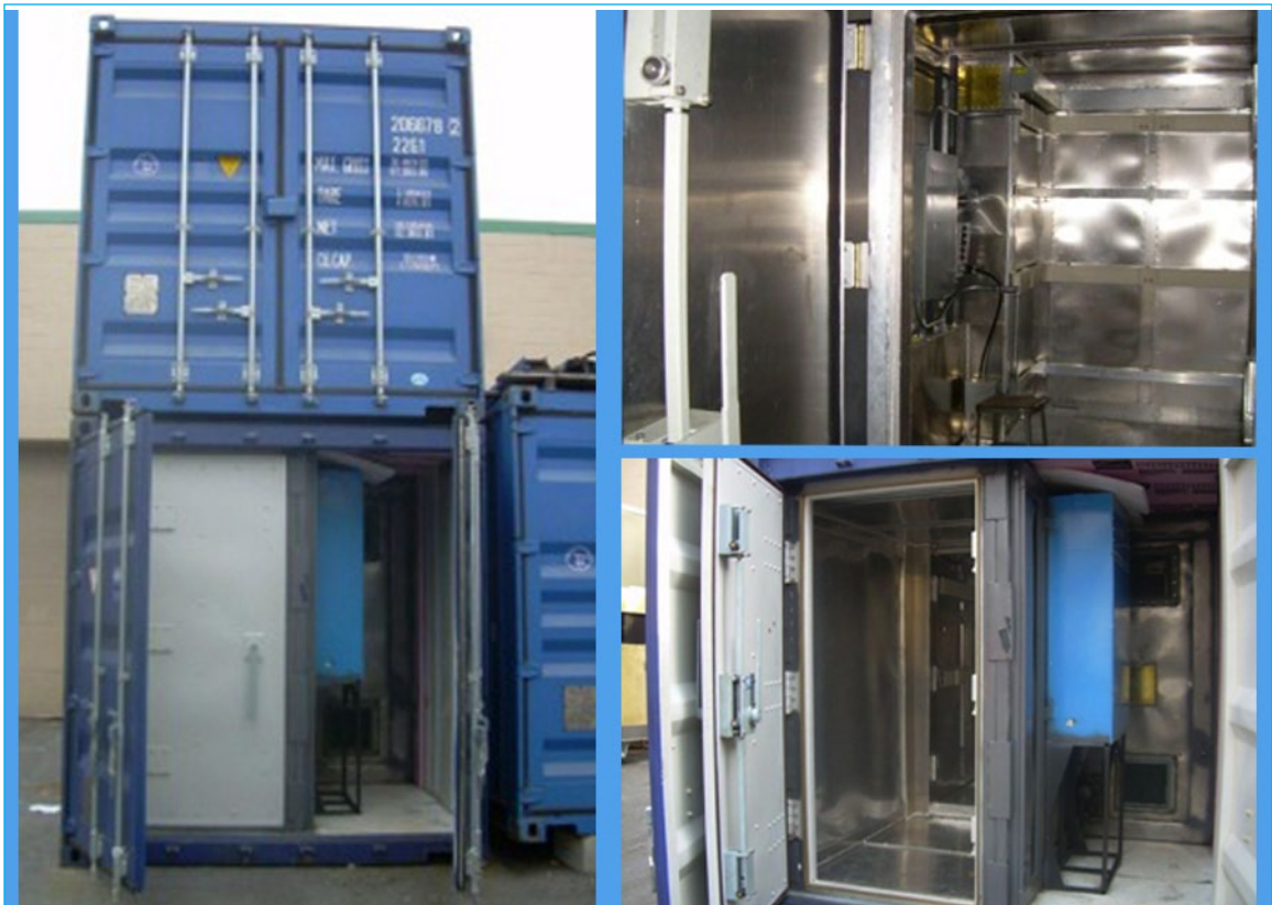
Figure 2: EMP-protected doors and filter systems as part of EMP protected 8x20 foot cargo containers.
