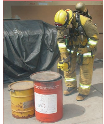
Bruker RAID-M Handheld Chemical Agent Detector with Lifeline Wireless capability in Hazmat response role.
