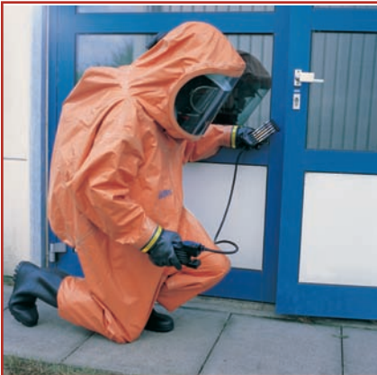
Dräger has developed a unique and important new detection system containing specialized sets that detect up to eight chemical substances, including nerve, blood and lung, nose and throat irritating agents in 5 minutes.
