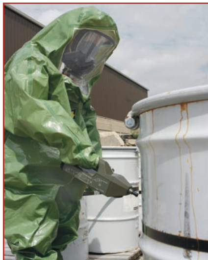
PROENGIN's AP4C simultaneously detects for Chemical Warfare Agents and TIMs/TICs.
