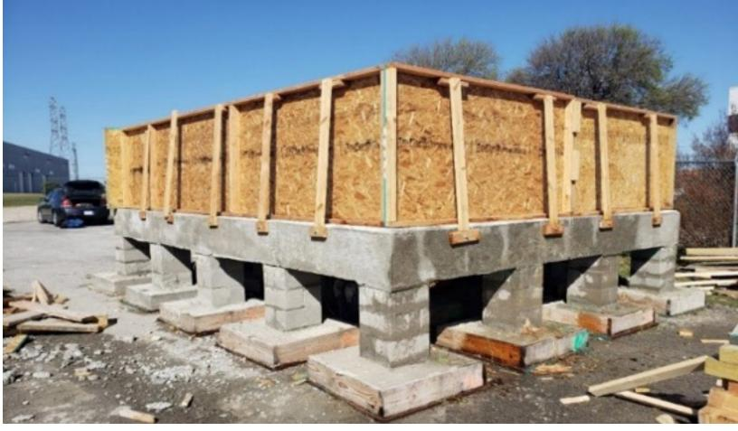
Fig. 1. Experimental two-way concrete slab with concrete masonry unit piers (Source: Authors, 2023).
